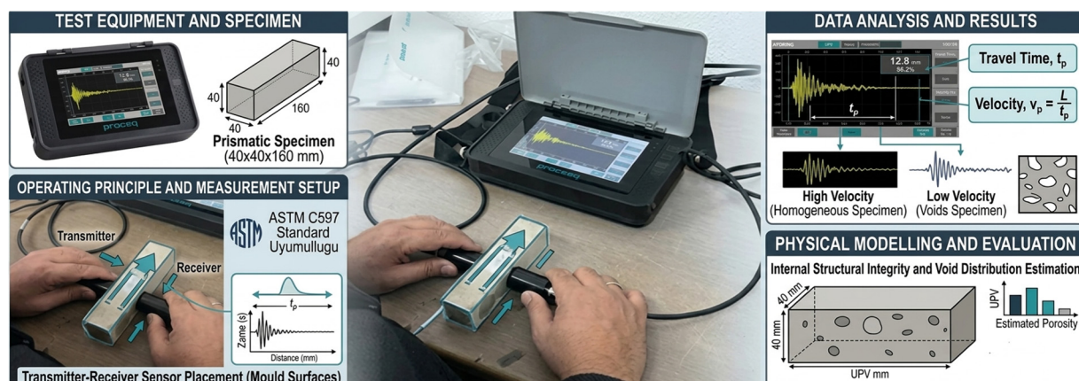
Figure 4. Proceq brand test device used for ultrasonic pulse velocity (UPV) measurement on geopolymer mortar samples.
