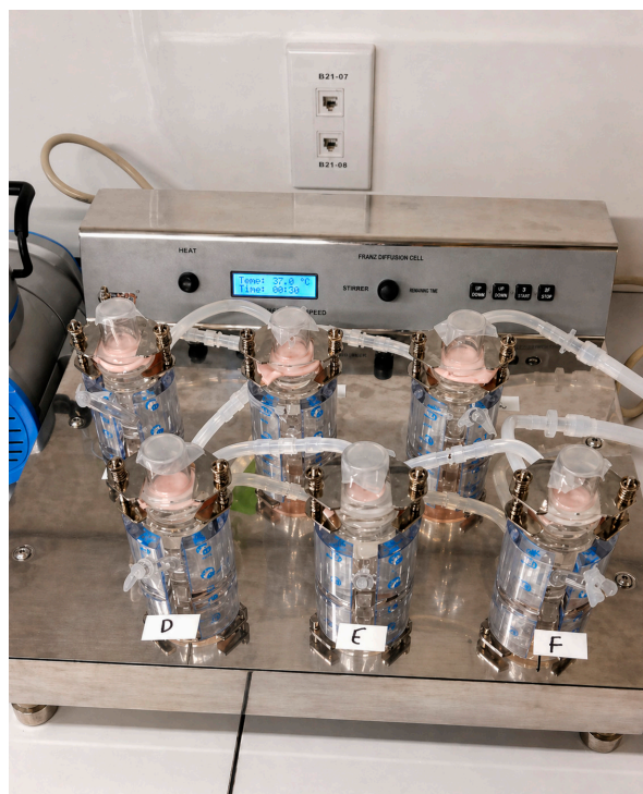
Figure 14. Setup of the ex vivo penetration using Franz cell.
