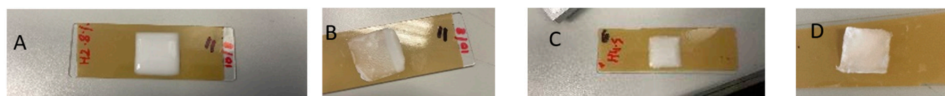
Figure 3. Effect of PEG concentration on the morphology of 3D-printed films before and after drying. (A) Film printed with 10% PEG before drying; (B) film printed with 10% PEG after drying; (C) film printed with 5% PEG before drying; (D) film printed with 5% PEG after drying.
