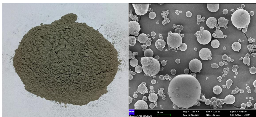
Figure 1. Physical appearance of fly ash and its SEM microstructure (1000×).
