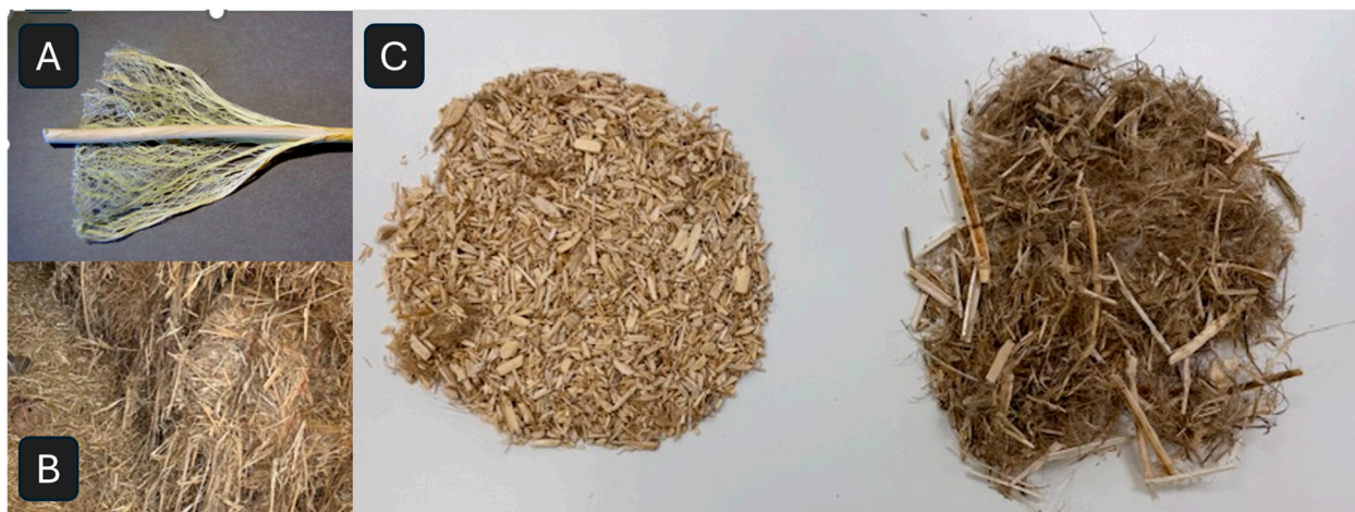
Figure 1. Photos depicting industrial hemp fibers, including (A) hemp stalks comprising both bast and hurd, (B) bales of air-dried harvested stalks with no processing or separation of fiber types, and (C) a comparison of processed, separated (decorticated) hemp hurd on the left versus minimally processed chopped hemp used in this study on the right. Chopped hemp is a mix of fine, longer outer fiber and coarser, shorter hurd fibers.
