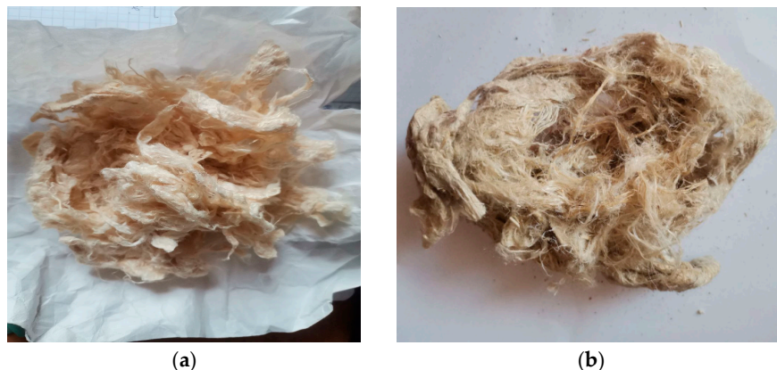
Figure 10. Cellulose fiber after alkaline (a) and after EHE (b) delignification.
