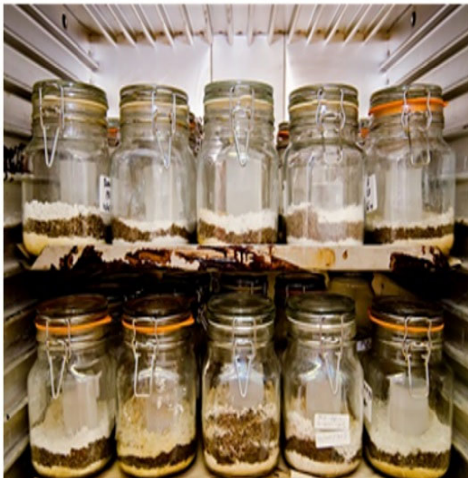
Figure 3. Soil and compost biodegradation testing at laboratory conditions.
