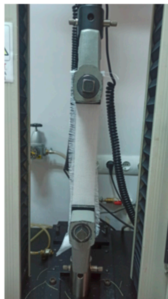
Figure 3. Tensile test of flax fabric sample.
