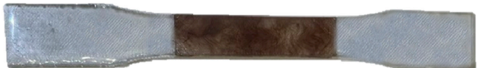
Figure 3. Tensile test specimen partial reinforced with jute fiber.
