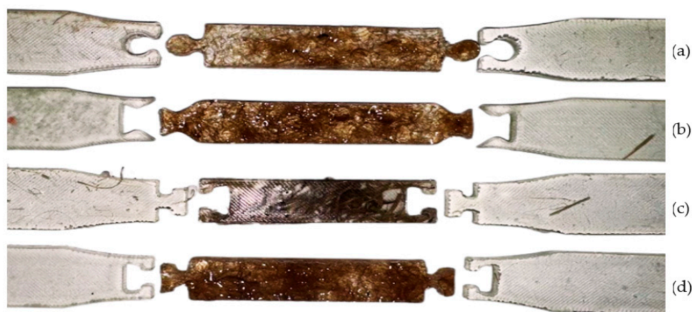
Figure 4. Segmentation of the tensile test specimen. (a) Puzzle, (b) dovetail, (c) T-channel1, (d) T-channel 2.
