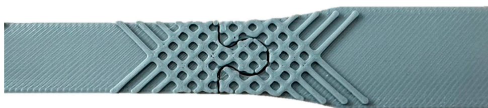
Figure 5. Another dimension—reinforcement using ribs.
