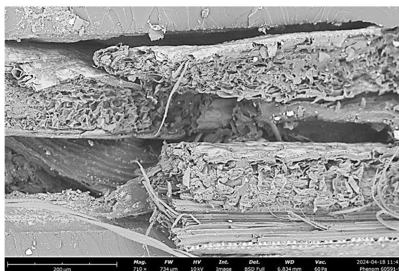
Figure 12. Microstructural analysis of 30% hemp fiber-reinforced polymer composites through SEM.
