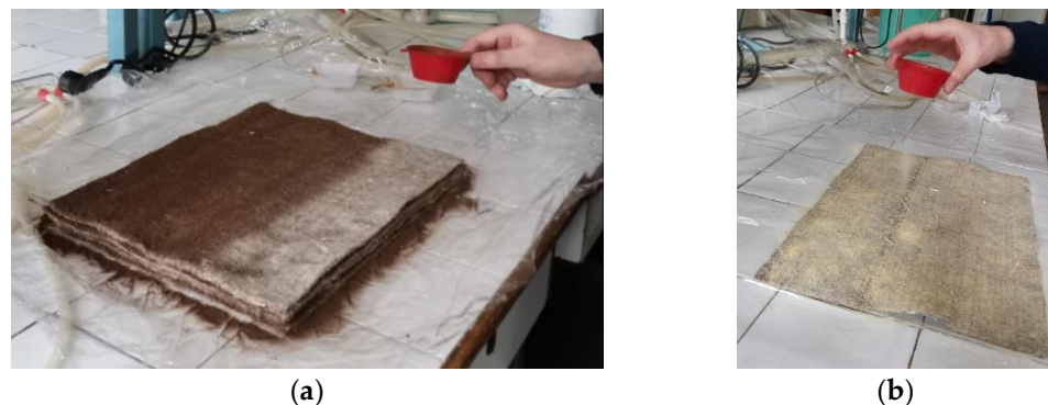
Figure 1. (a) Soda lignin sieving; (b) lignosulfonate sieving on the nonwoven pieces.
