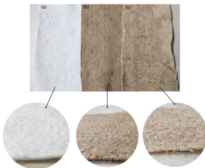
Figure 1. The nonwoven mulch blends with 20% of PLA fibres and (a) 80% of viscose, (b) 80% of jute, (c) 80% of hemp fibres.
