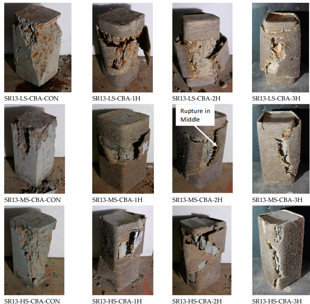
Figure 13. Ultimate failure pattern of low-strength, medium-strength, and high-strength square specimens with and without confinement.
