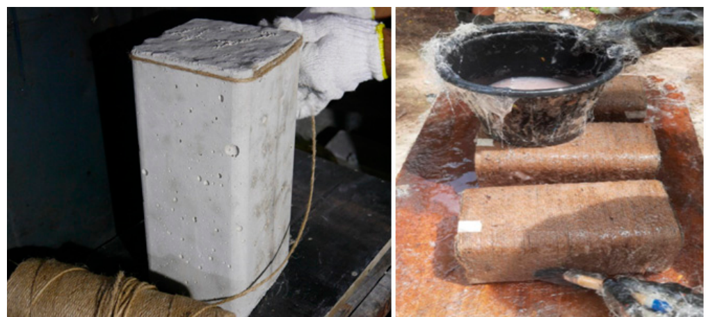
Figure 6. Application of two-part epoxy and fiber ropes to square specimens.
