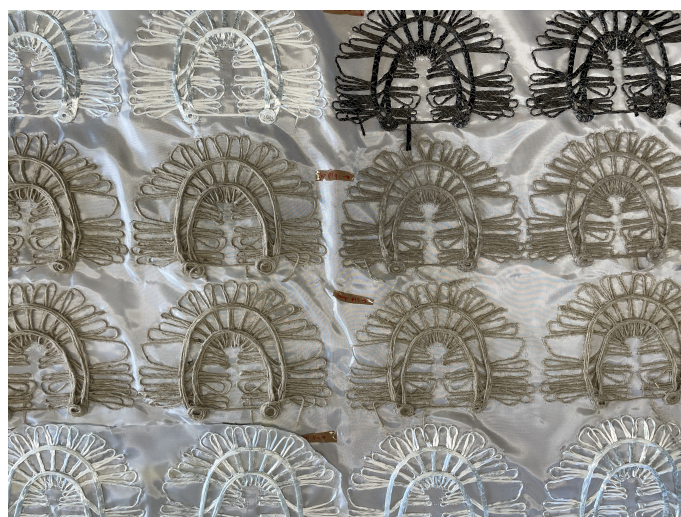
Figure 4. Preforms manufactured by TFP and made of different roving materials: glass, basalt, flax, and jute.
