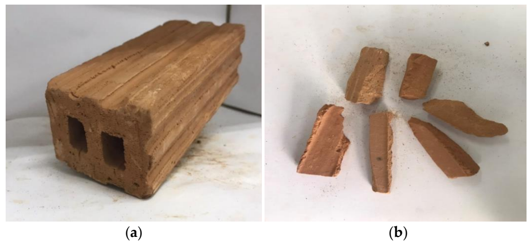
Figure 3. (a) Fired-clay interlocking bricks and (b) aggregate obtained from fired-clay interlocking bricks.
