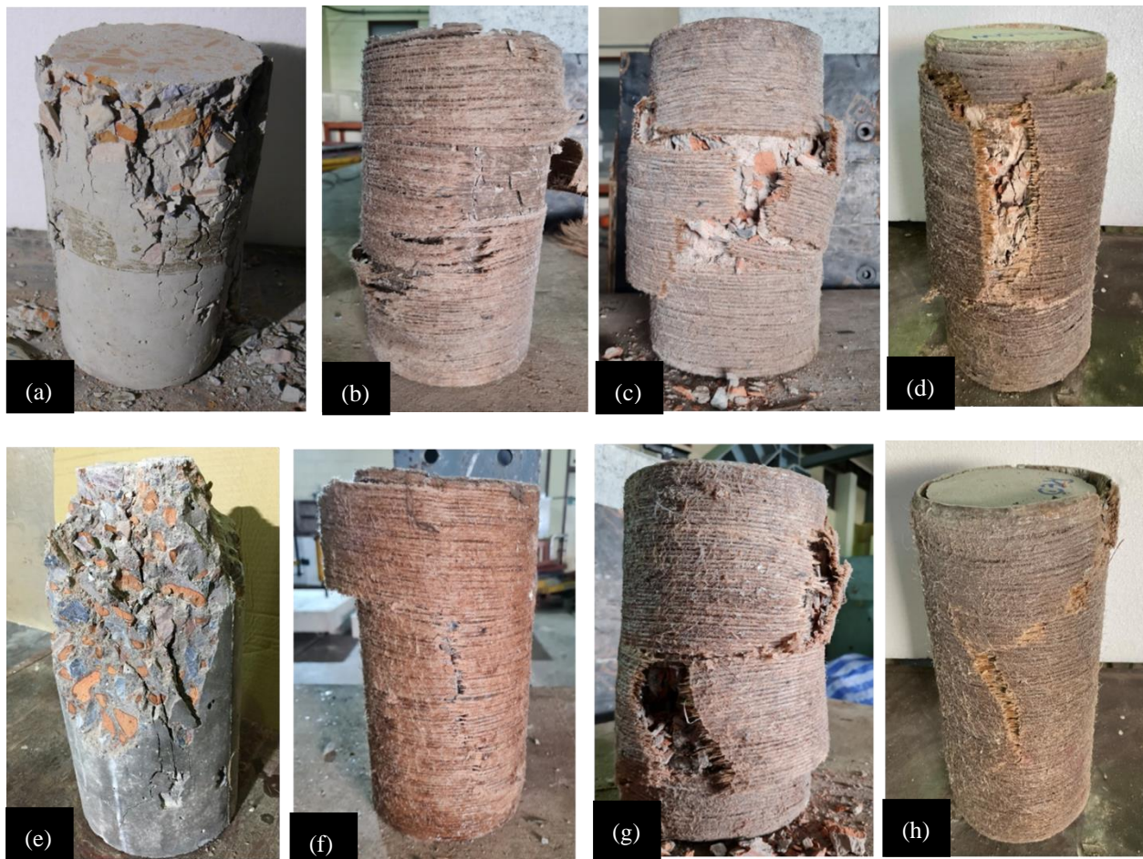
Figure 11. Ultimate failure pattern of specimens: (a) C-LS-CBB-CON, (b) C-LS-CBB-1H, (c) C-LS-CBB-2H, (d) C-LS-CBB-3H, (e) C-HS-CBB-CON, (f) C-HS-CBB-1H, (g) C-HS-CBB-2H, and (h) C-HS-CBB-3H.
