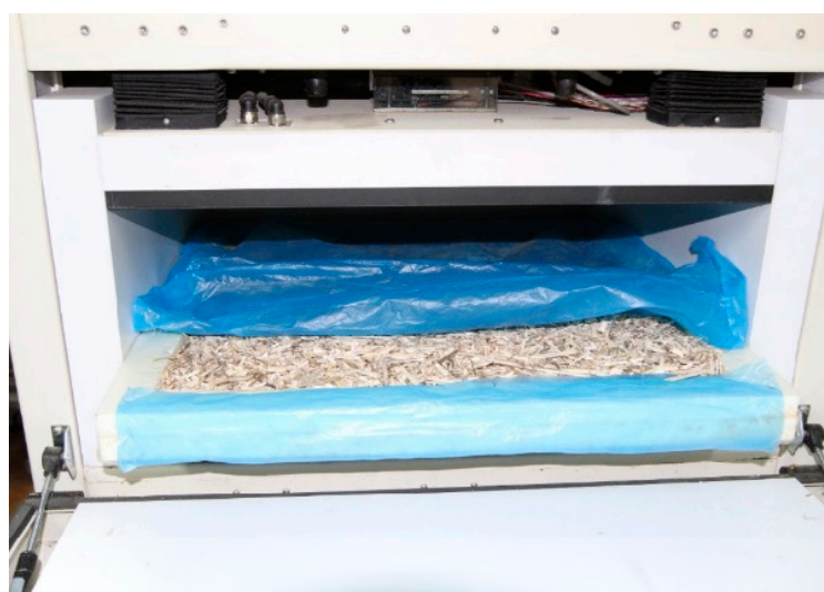
Figure 2. A prepared sample of dry HS placed in the HFM apparatus [29].
