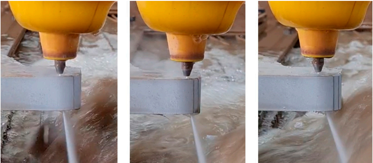
Figure 6. Example view of AWJ cutting process with different deflection angles.
