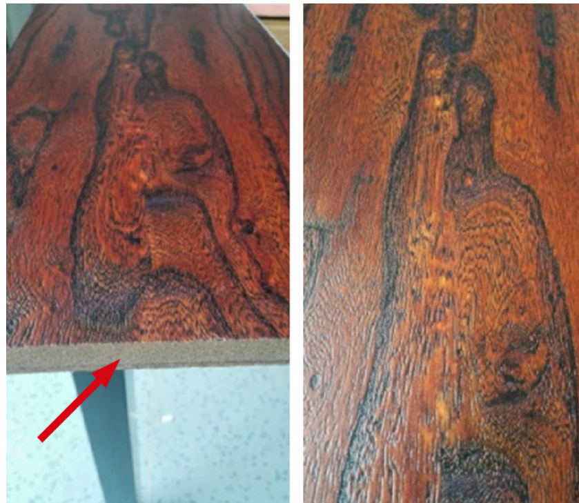
Figure 9. An example of a primary application for WPCs: direct-to-substrate 3D printing to create a realistic elm wood texture. The red arrow indicates the substrate material onto which the texture is printed. The technical conclusion this illustrates is that the main engineering driver for WPC use is often aesthetic and cost-reduction, rather than structural reinforcement. Research consistently shows that wood flour typically acts as a filler, which can significantly reduce mechanical strength compared to the neat polymer. This positions WPCs as an ideal material for non-structural, decorative applications like the one shown [192].
