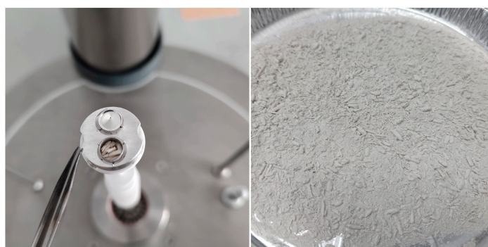
Figure 5. Hemp shiv sample in DSC crucible and example crushed sample of hemp-lime composite prepared for specific heat testing.
