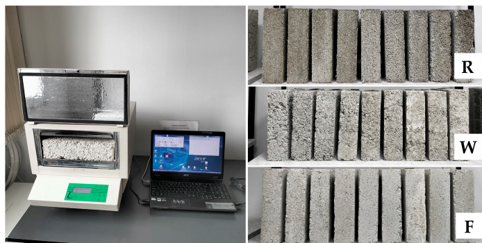
Figure 3. Fox 314 apparatus and samples of all series prepared for thermal conductivity tests.
