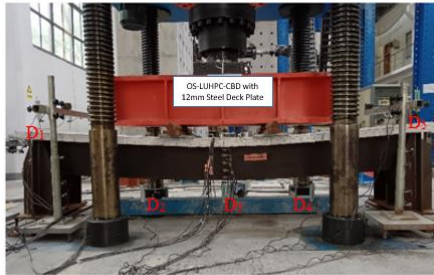
Figure 11. Dial indicators marked D 1 to D 5 installed to measure vertical deflections.
