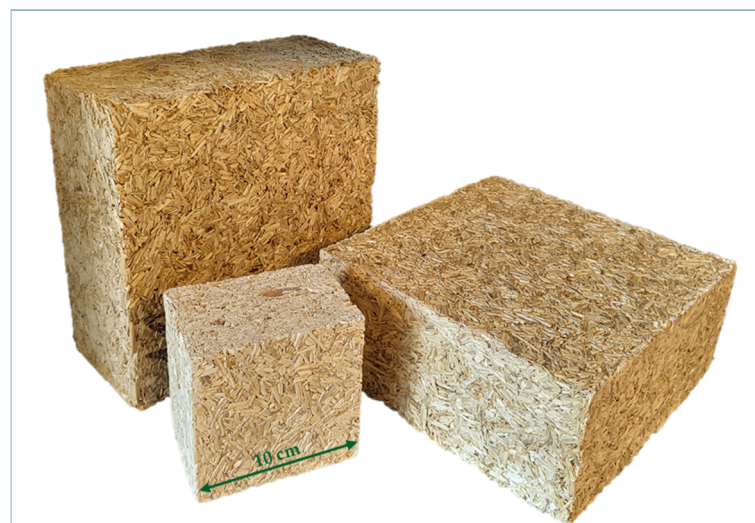
Figure 5. The obtained bio-composites bounded by potato starch binder.
