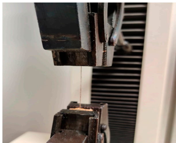
Figure 2. Fiber in the handles of the testing machine.
