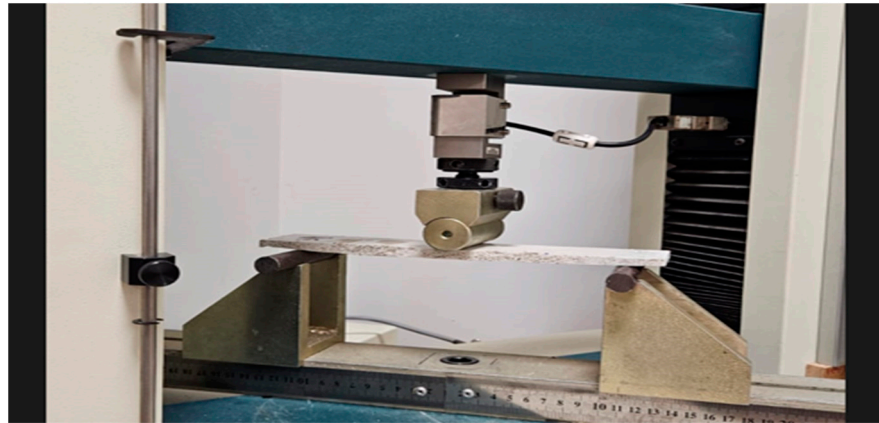
Figure 3. Measurement of mechanical characteristics in the 3-point bending test.
