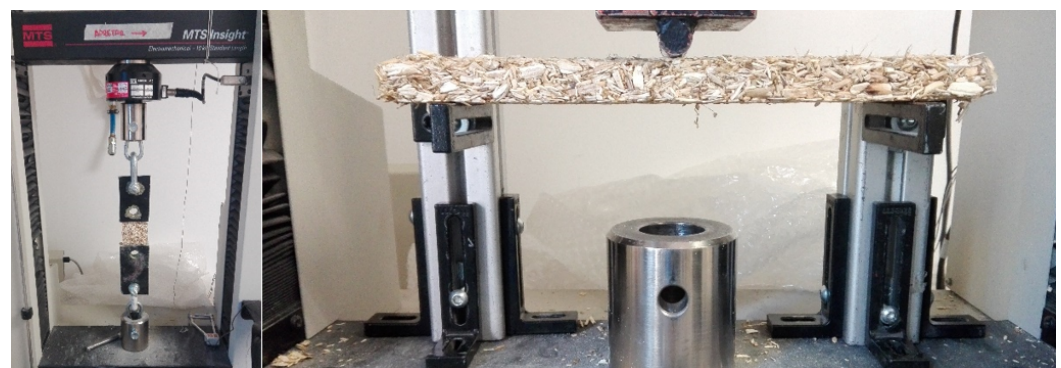
Figure 3. Test configuration: tensile (left) and bending (right).
