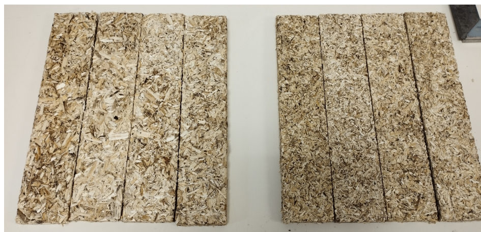
Figure 2. Specimens made with arabic gum.
