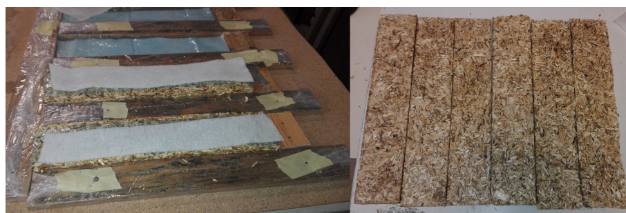
Figure 4. Wooden mold with bleeding and absorbent paper (left) and obtained specimens (right).
