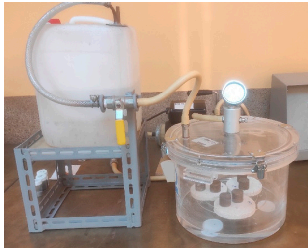
Figure 5. Sample vacuuming process.
