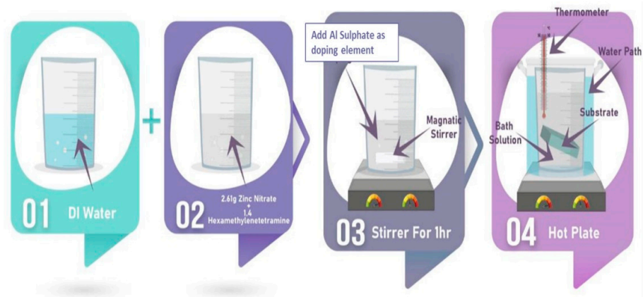
Figure 2. The steps followed for the preparation of AZO via CBD approach.
