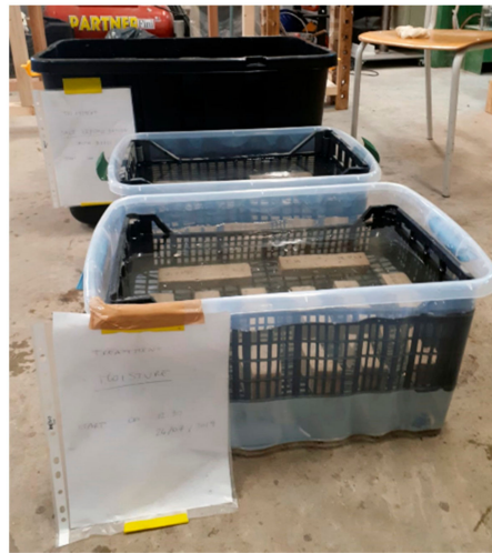
Figure 4. Specimens immersed in exposure environments: the saltwater environment in the black tank, moisture environments in white tanks.
