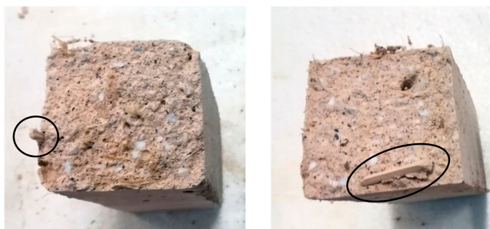
Figure 10. Examples of agglomeration of hemp fibers in tested specimens.
