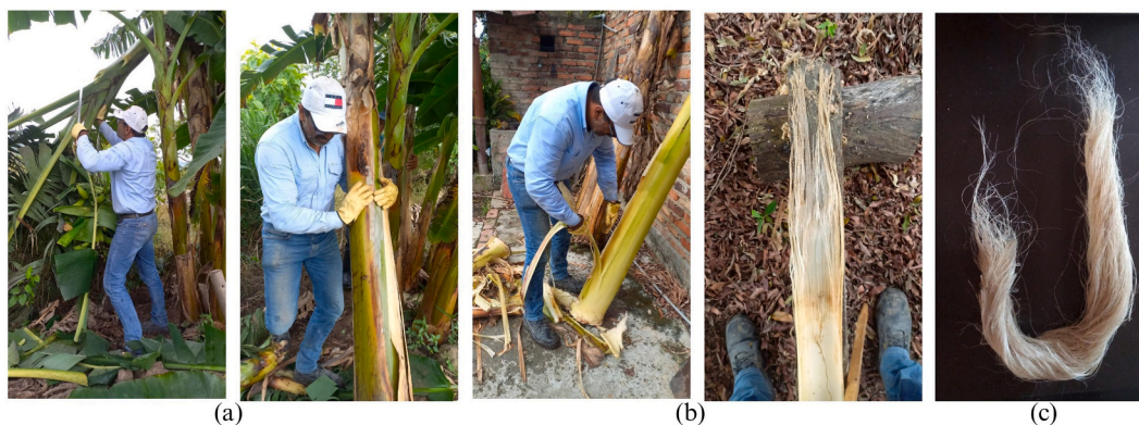
Fig. 4. Plantain pseudostem fibers extraction process. (a) Cutting of plantain bunch and pseudostem. (b) Manual fibers extraction. (c) Extracted fibers.
