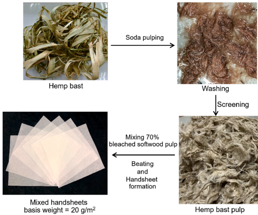
Fig. 2. Preparation of hemp bast handsheet samples.
