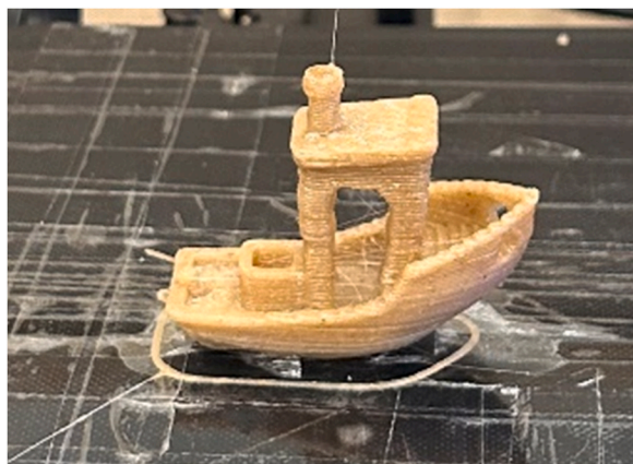
Fig. 2. Additively manufactured 3D benchy using PPHF composite material.
