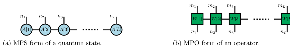
Figure 2. Graphical tensor network representation of an MPS and MPO. The logical wave function and operator are obtained by contracting the matrices A[i]^{n_i} and W[i]^{m_i} , respectively.
