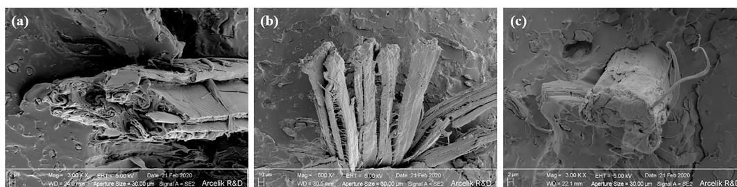
Figure 5. SEM images of (a) nonpretreated, (b) alkaline-pretreated, and (c) silane-pretreated wH.
