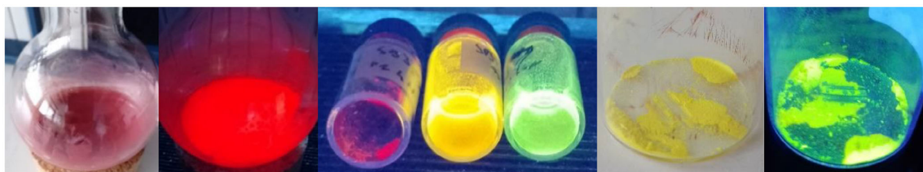
Figure 12. Images of the red (round flask, left) and yellow (powders, right) solids of [PtLHCl] under ambient condition and UV irradiation ( \lambda_{\text{Exc}} = 366 \text{ nm} ). Pure red solid of [PtLHCN] obtained from DCM (center-left), suspended in EtOAc (yellow suspension, center), and in an EtOAc/MeOH-mixture (center-right) for 10 min observed under UV irradiation ( \lambda_{\text{Exc}} = 366 \text{ nm} ).
