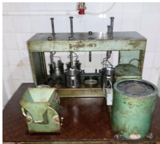
FIGURE 10 | Oil extraction system (oleodoseur) used at the Technical Institute of Fruit Arboriculture and Vineyards (TIFAV), Sidi-Aiche, Algeria. All images are original and were created by the authors for this manuscript.
