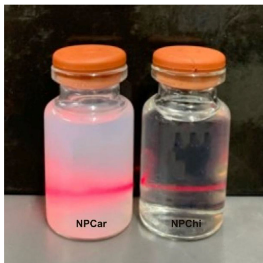
FIGURE 2 | Samples of the nanoformulation of chitosan (NPChi) and chitosan nanoparticles containing Car (NPCar).
