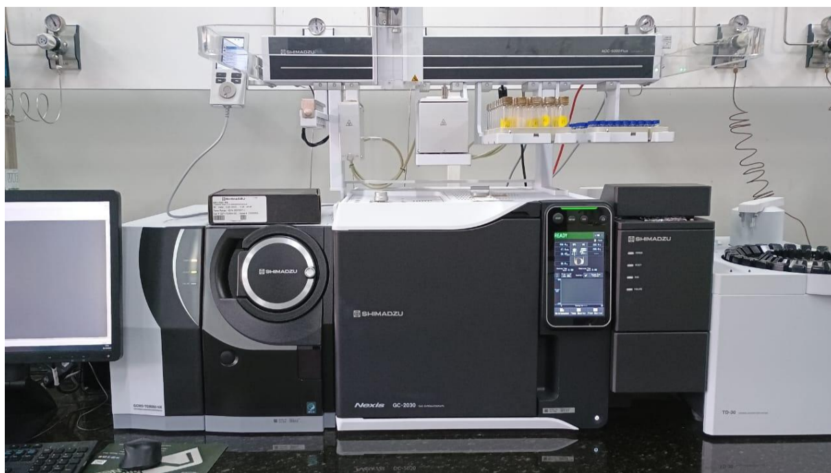
Figure S4. Shimadzu GC-2030 gas chromatograph coupled to a GCMS-TQ8050 NX mass spectrometer.
