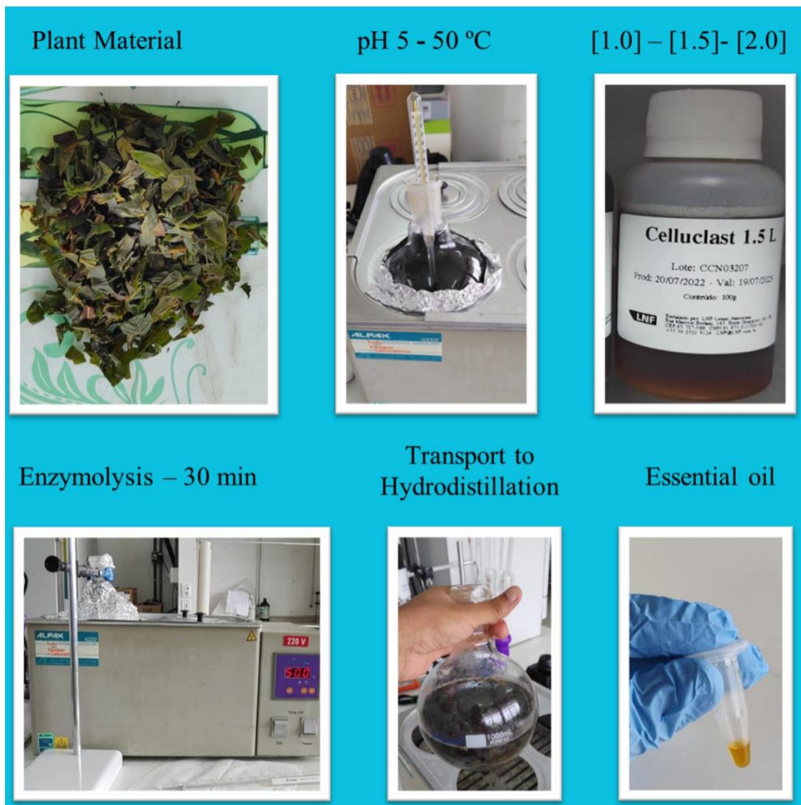
Figure S3. Graphical cellulase-assisted hydrodistillation method.
