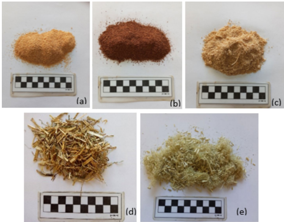
Fig. 1 Utilized bio-materials (a) black pine wood powder (BG), (b) black pine bark powder (BB), (c) pellet crumb (P), (d) agro-pasture fibers (A) and (e) hemp fibers (H)
