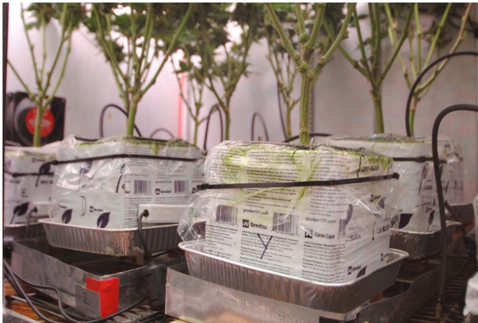
Fig. 1 Cannabis ‘Trump’ growing in stone wool on load cells. Plastic wrap covered the tops of stone wool to minimize evaporation
