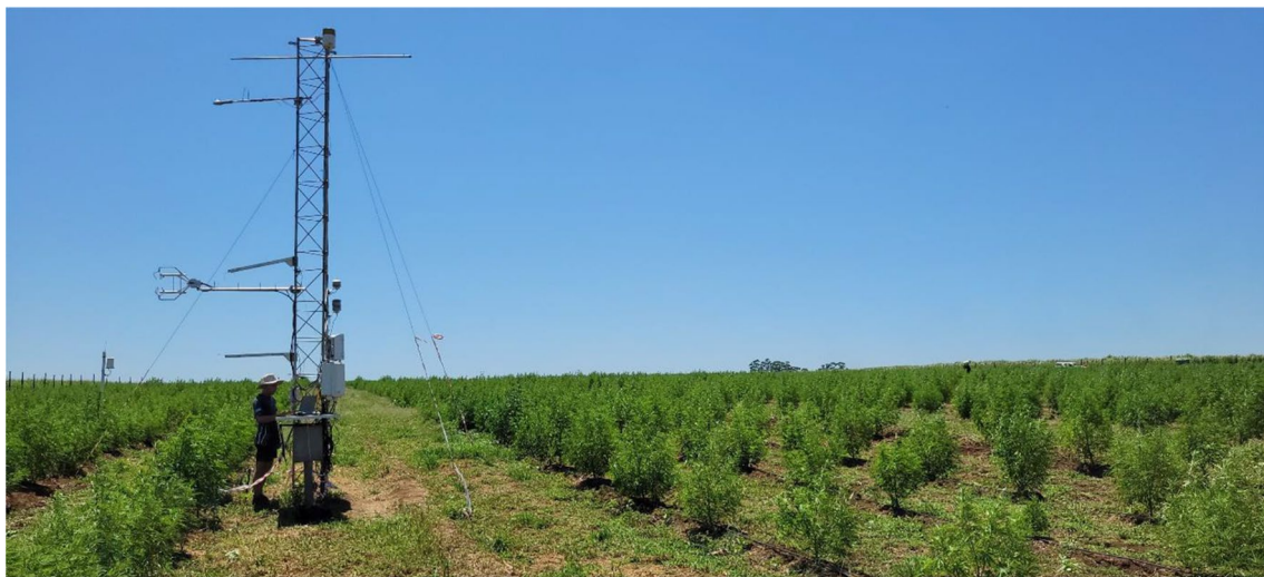
Plate 2 Tower and eddy covariance system measuring evapotranspiration on 24 January 2023
