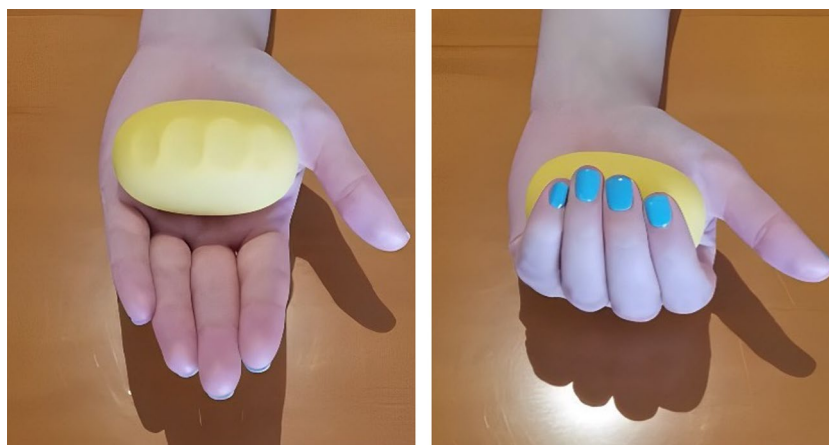
Figure 3. Squeeze ball dynamometer (Smart Stress Ball, 2019 China) used by participants to record daily grip strength to their smartphones via Bluetooth.
