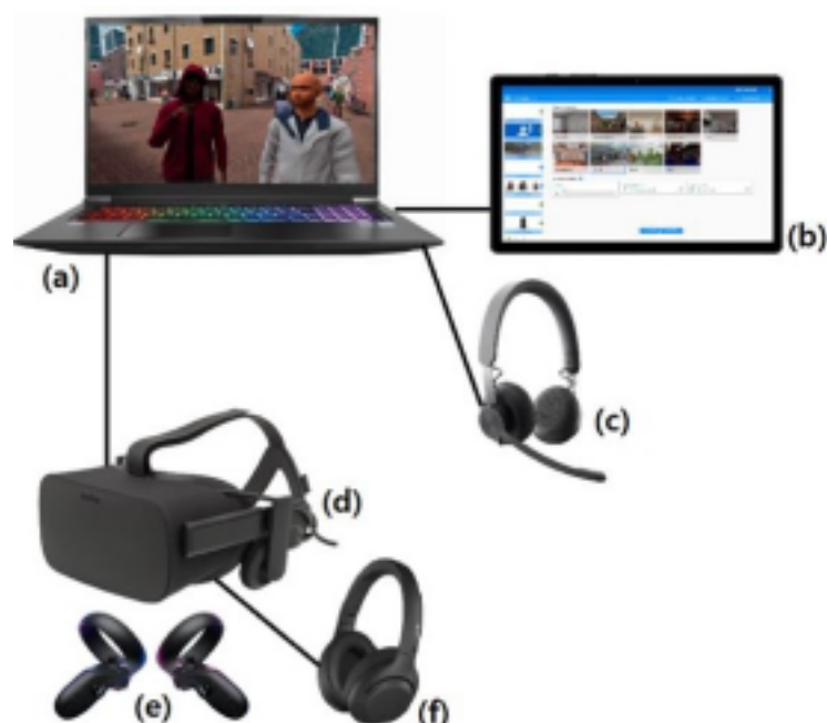
Fig 3. Setup of VR technology consisting of a laptop (a), a tablet with the dashboard (b), a voice-morphing microphone (c), a VR head-mounted display (d), VR controllers (e), and
