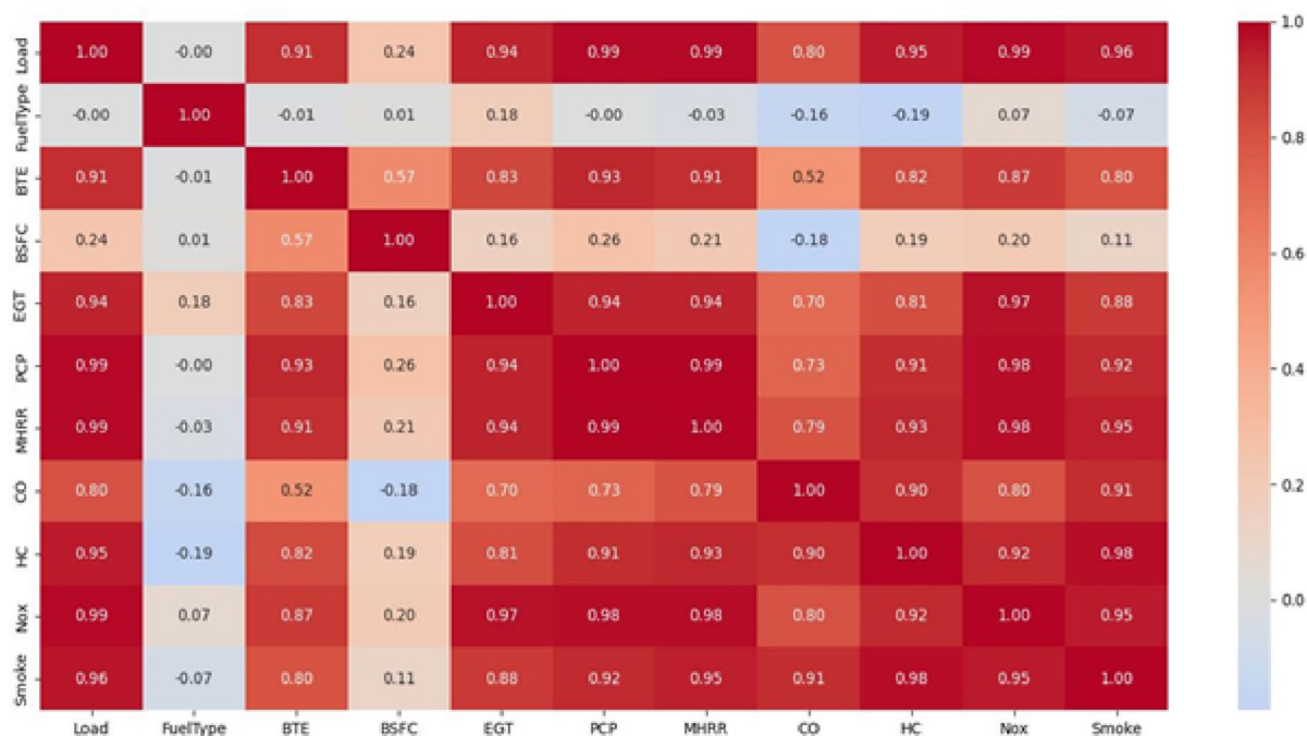
Fig. 28. Correlation heat map for all engine parameters.
