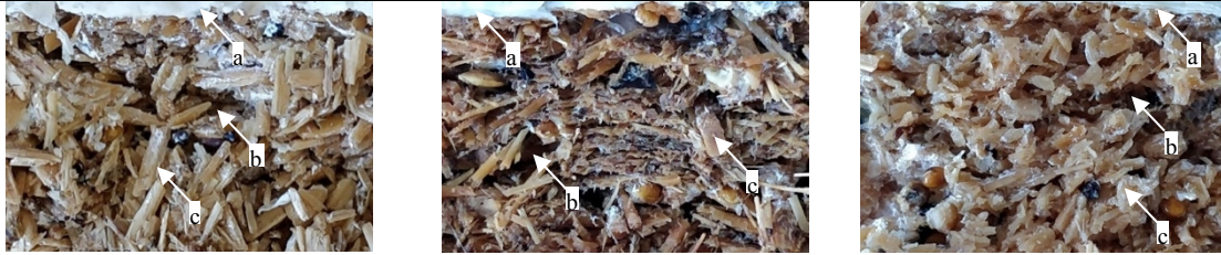
Figure 6: Cross section of the inner growth of undried FL, FWL and FL samples. (a) mycelium chitinous layer, (b) air-void, (c) limited decayed fibre by mycelium.
