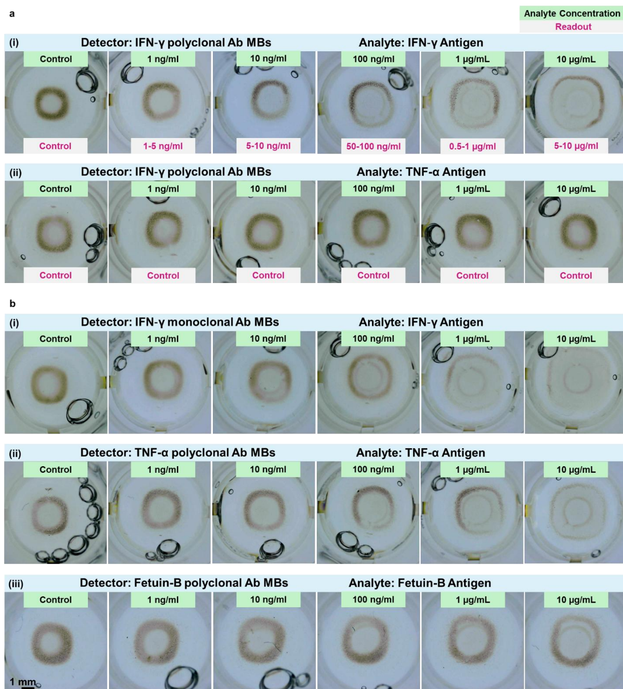
Figure 5. SIMAIS platform performance evaluation. a, Specificity/ selectivity. MBs functionalised with IFN- \gamma polyclonal antibodies are tested with serial dilutions of either on-target IFN- \gamma antigen (i) or off-target TNF- \alpha antigen (ii). The ML classifier correctly assigns each on-target sample to its concentration level, while labelling every off-target well as “Control”, confirming negligible cross-reactivity. b, Transferability to other antibody-antigen pairs. MB pattern trends are reproduced with alternative detectors: (i) IFN- \gamma mAb-
