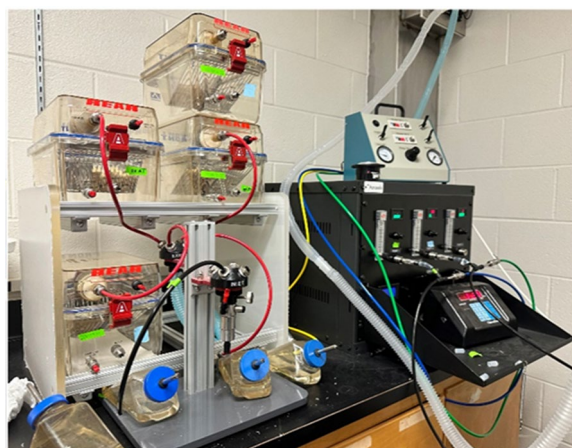
Fig. 1 Automated vaping exposure system. A prototype of an automated exposure system (CSM-eSTEP) that includes an e-cigarette puffing machine, developed for small-scale inhalation exposure. In this study, we used the CH Technologies Modular BCU Exposure Chamber that are ideal for small-scale whole-body exposure studies. We adopted the Electronic Cigarette Aerosol Generator (ECAG) platforms that are designed specifically for electronic cigarettes and all vape products from the ground up. Here, instead of vaping liquids, e-cigarette cartridges were filled with CBD solution. This novel positive pressure system allows for more accurate physicochemical characterization and delivery at the exhaust port, reducing aerosol aging, and tube deposition, and eliminating artifacts that could be introduced from background air. The ECAG was designed to accommodate one-piece disposable electronic cigarettes (i.e., cig-alikes), in addition to the refillable tank/clearomizer 2nd thru 4th generation devices. CBD aerosols were generated from electronic cigarette (E-Cig) cartridges filled with 1 ml of CBD solution instead of vape fluid. CH Technologies aerosol generator generated CBD puffs (10 puffs for every 5 min, which repeated every 25 min up to 2 h)
